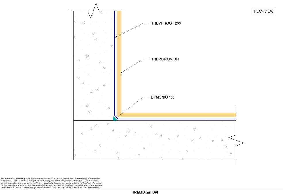
Detail: TREMDrain DPI with TREMproof 260 at Inside Corner
